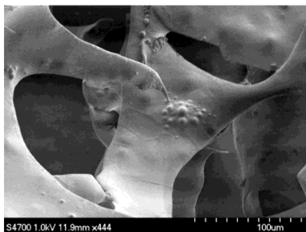
Figure 8 Low- and high-magnification SEM micrographs of liberated LDPE films collected near the inner cylinder for N = 23 .
